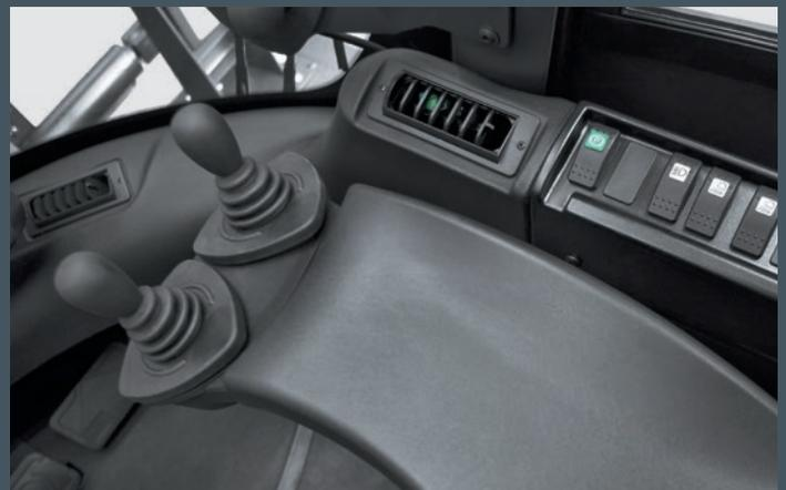
Fully adjustable suspension seat and integrated armrest incorporating the fingertip Linde Load Control, integrated in an adjustable armrest for effortless and secure load handling.
