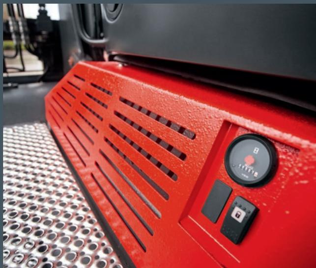
The main chassis structure has been coupled directly to the counterweight structure, which is designed to absorb vibration; the steering axle is directly mounted into the counterweight by resilient cushioning, thereby absorbing travel shock and vibration.
